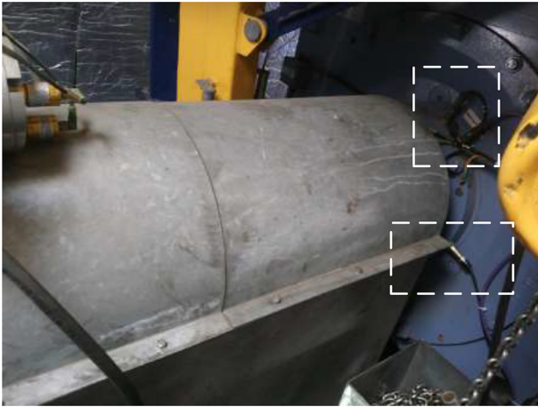
Fig. 8. Installed location of vibration accelerometers. (The accelerometers are mounted on outside of the generator in wind turbine horizontally and vertically, respectively.).
