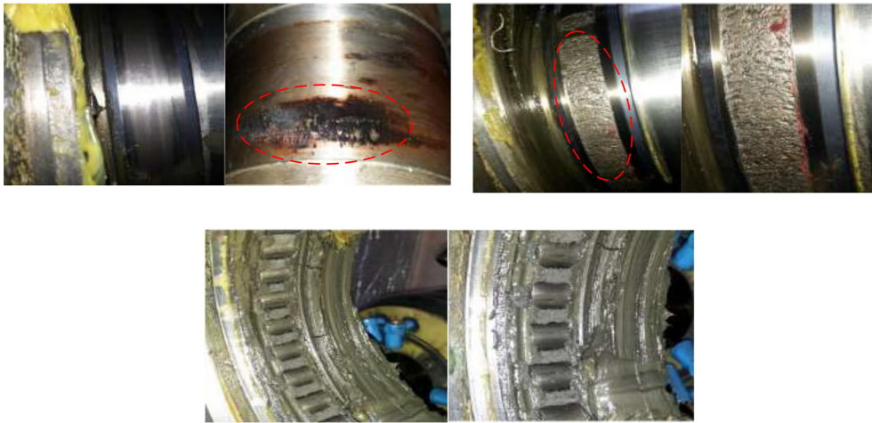
Fig. 17. Failures in inner race of rolling bearings (The regions of the dotted line are the defect with worn inner race).
